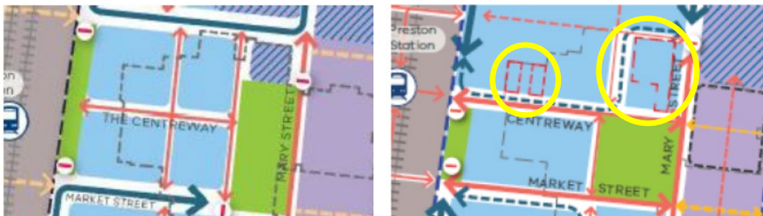
Figure 30 Access to private property (circled yellow) maintained with PMD north loop road (VPA plan on the left)
