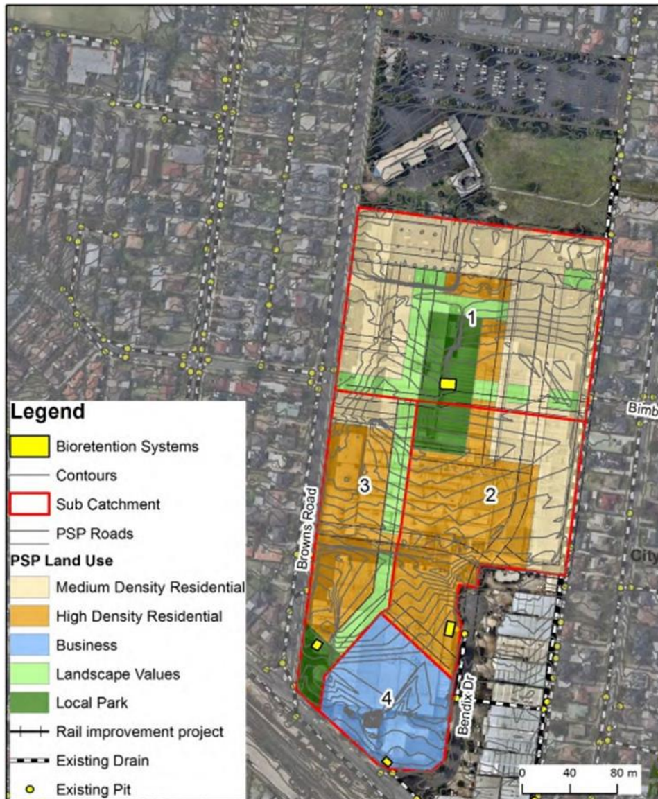
Figure 13 Stormwater treatment preferred option Scenario 1 - End of catchment WSUD assets
