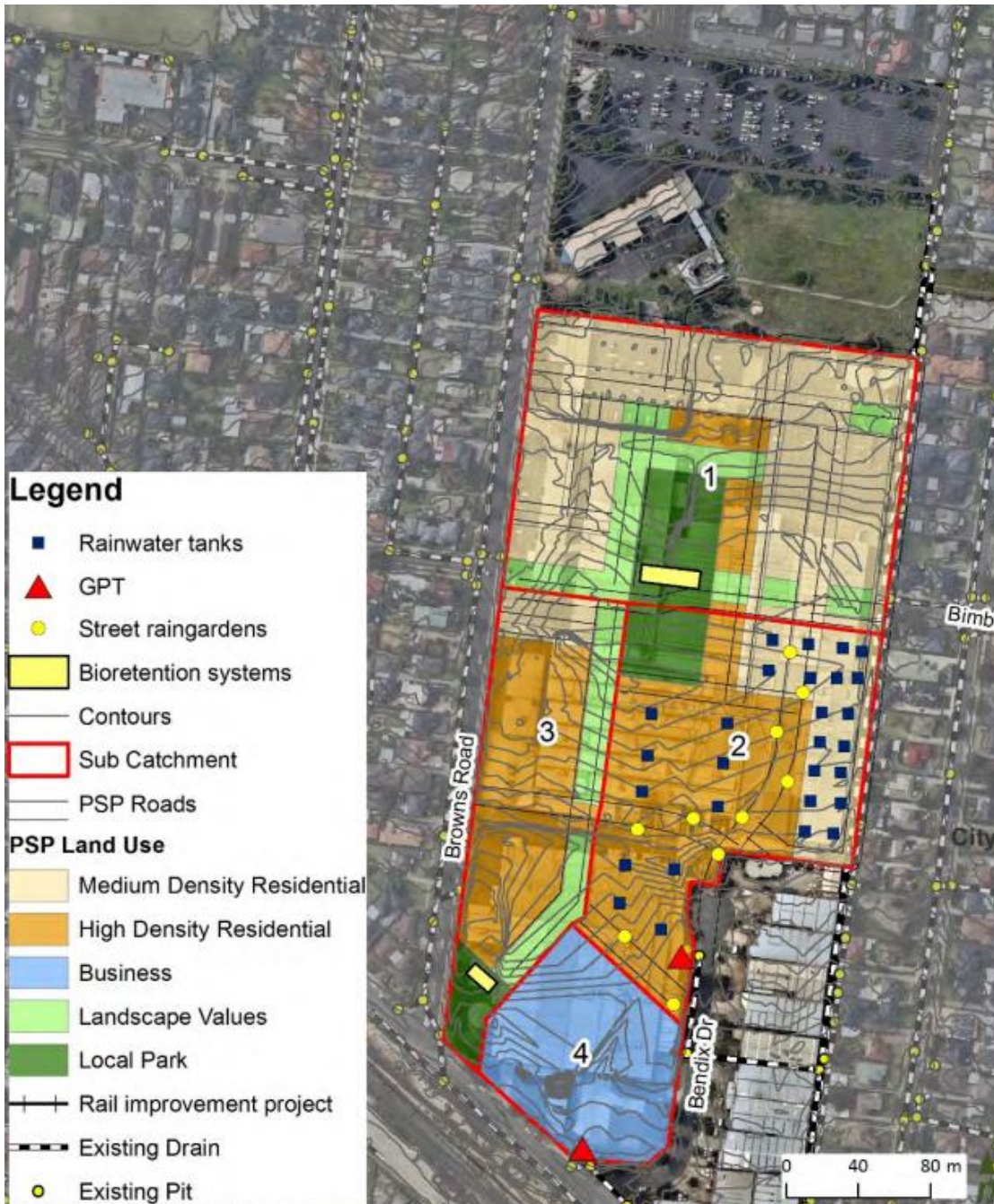
Figure 15 Stormwater treatment Scenario 3: Oversized WSUD in open space with rainwater reuse and distributed WSUD in sub-catchments 2 and 4.
