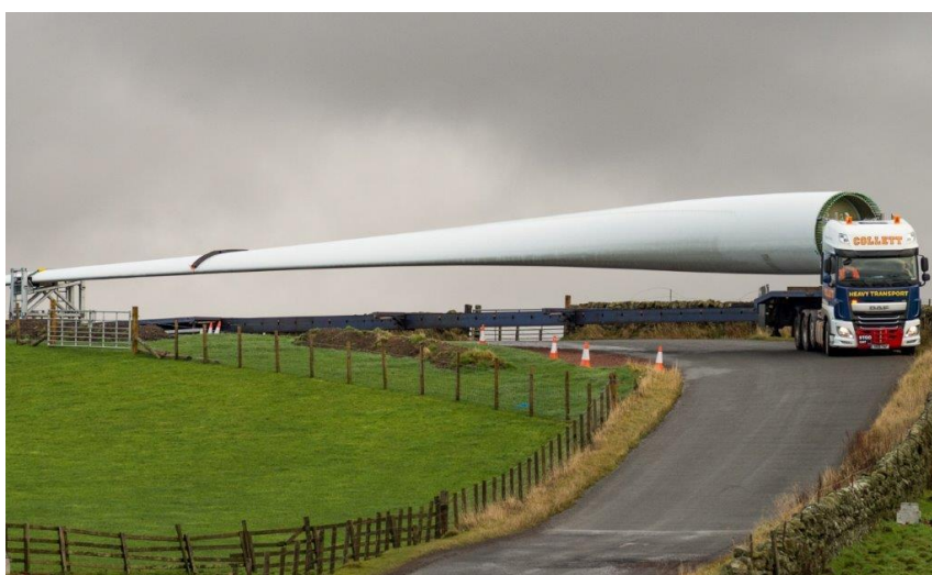
Figure 11 Photograph of a turbine blade being delivered to a wind farm site Source: Traffic Impact Assessment by GTA Consultants, page 9
