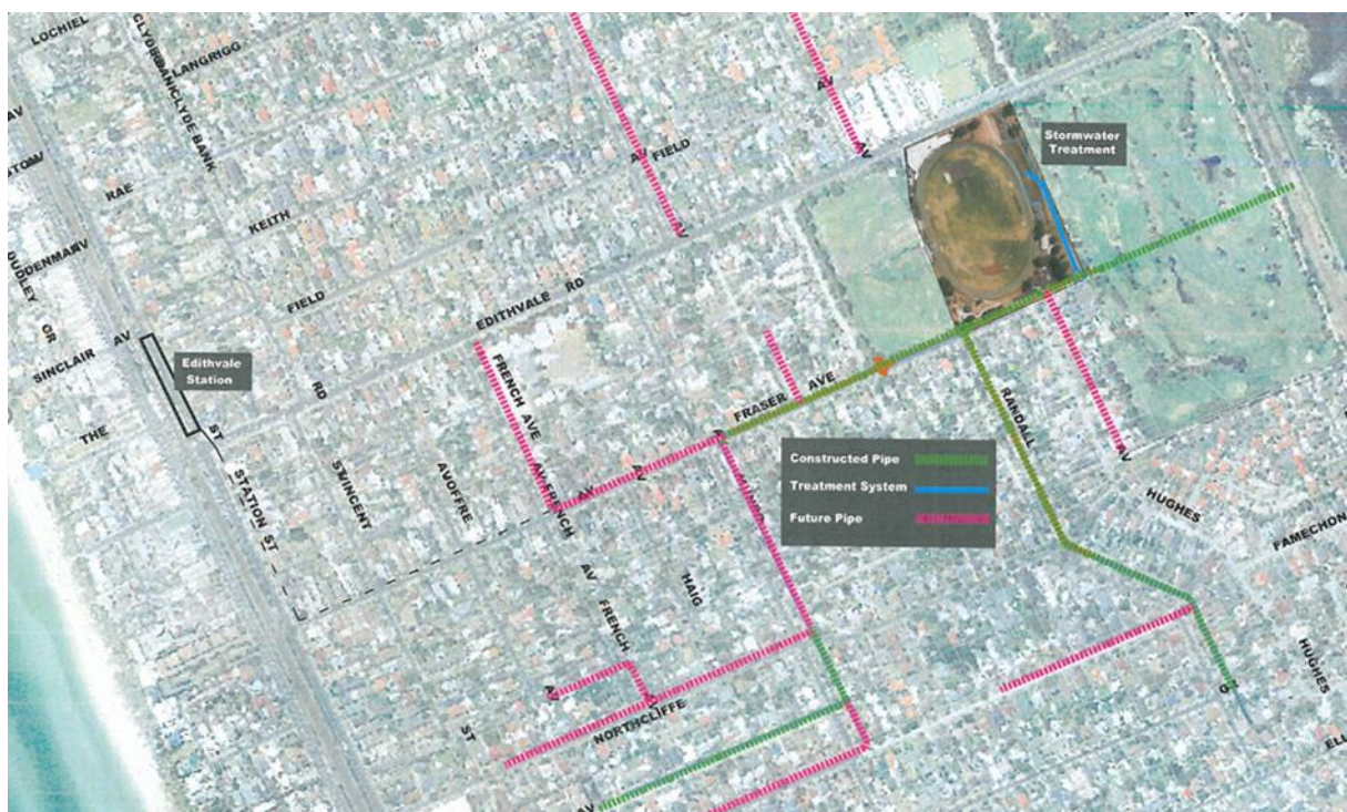
Figure 7 Edithvale Project – surface water drainage scheme (Source: Document 23, Council)
