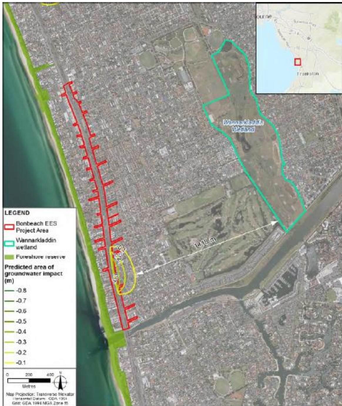
Figure 17 Extent of groundwater change post-trench installation at Bonbeach (inland) 157
