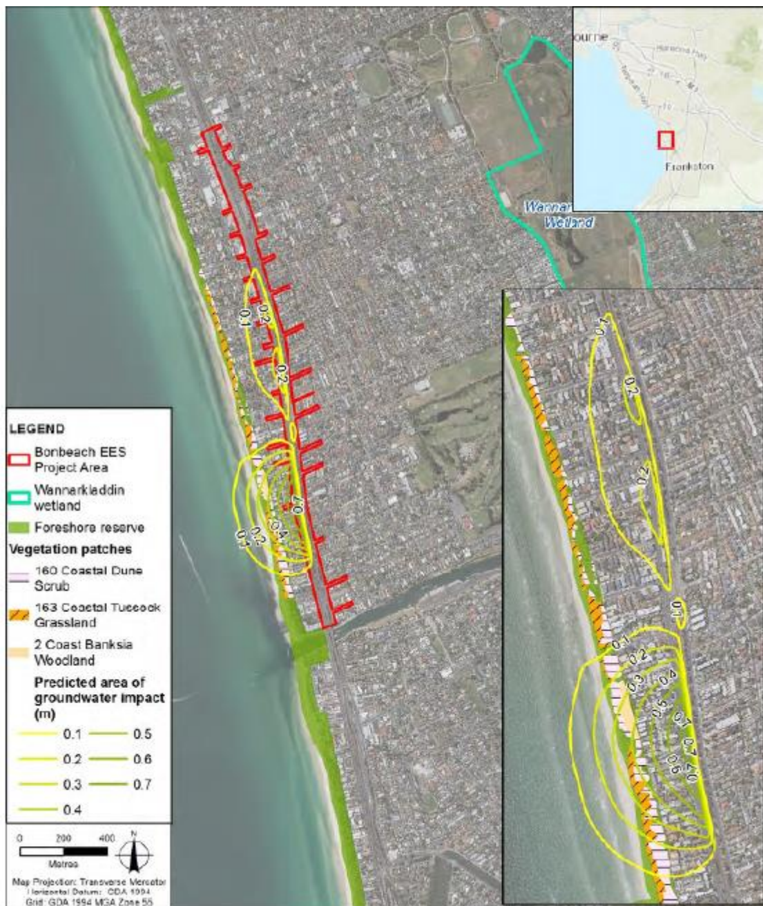
Figure 23 Extent of groundwater change post - trench installation at Bonbeach (coastal)
